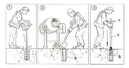
(A) Rubble (B) Taper (C) Self-drilling screws (D) Dave the Installer(E) Item/ Installation Tool (F) Spirit Level (G) Concrete 30 MPa
